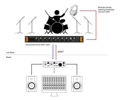
This is how larger recording studios are set up: the recording engineer is in one room and one or more musicians are in another room, on the other side of a window. The AudioFuse 8Pre is being used as a multi-channel direct box, a high-quality A/D converter, and also as a headphone monitoring system for the drummer.
