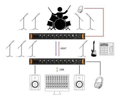
Two AudioFuse 8Pre units are connected through a pair of optical cables. A USB cable connects the first unit to the computer, which sees the two units as if they were a single 16-channel input device. The drummer is listening to the master mix through the headphones, with the monitor section of the nearest AudioFuse 8Pre set to Main 1-2.
