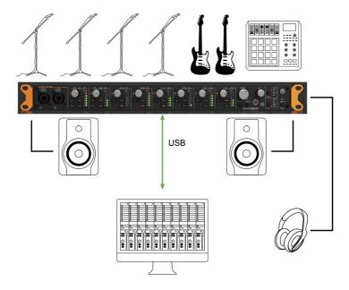
In this scenario the AudioFuse 8Pre is the only audio interface. Its eight analog inputs are being used several ways:
