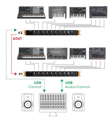
Synth lovers, this one is for you! Here we have two AudioFuse 8Pre units, and each one is connected via USB to the same computer. A single ADAT optical cable connects the two AudioFuse 8Pre units, with AudioFuse 8Pre #1 in USB mode and AudioFuse 8Pre #2 in ADAT mode.
