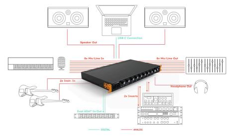
Eight of those inputs and outputs can be provided through optical cables by another ADAT-equipped device, such as another member of the AudioFuse family.
