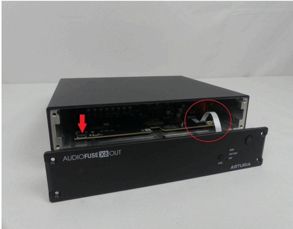
*The USB-C type connector is on the left hand side.*
