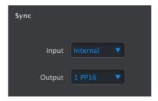
These settings allow you to specify the inputs for receiving synchronization and tempo signals, as well as the input and output clock rates. By changing these settings, you determine which type of clocking signal will be transmitted via the output connectors and which type will be recognized by the sync/clock inputs.
