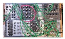
Another interesting use of the KeyStep Pro is as the master clock of your Eurorack modular or RackBrute system. To make this possible, the KeyStep Pro has a Clock Output. A smart solution is to connect the KeyStep Pro's Clock Out to a clock divider, which will divide the tempo in half or smaller fractions. You can then use these timing signals to start events on each beat, every other beat or each bar, for example.
