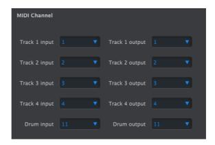
In this menu, you set the Global channels on which the four tracks of the KeyStep Pro will send and receive MIDI signals. The four tracks default to their track number (MIDI channels 1-4); the Drum channel defaults to MIDI channel 10.
