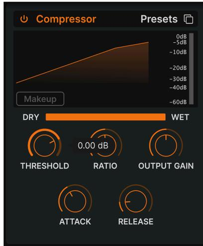
A **Compressor** is used to control the dynamic range of a sound: it reduces the difference between the softest and loudest levels a sound can have. It does this based on reducing a gain by a certain amount (the ratio) once the audio releases a certain level (the threshold).
