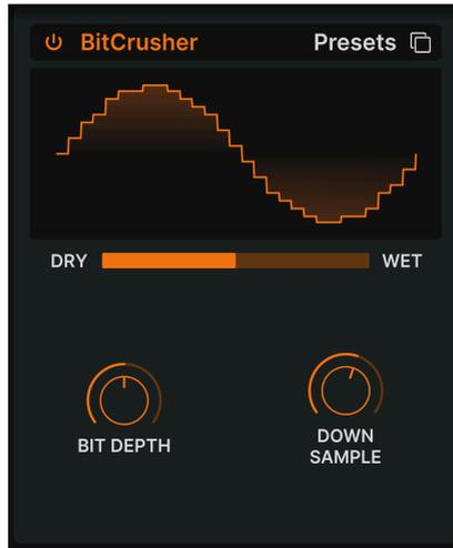
A **bitcrusher** does exactly what it sounds like: it crushes bits! Technically, it can reduce both the bit depth and the sample rate of the signal. Bit depth (e.g. 16-bit vs. 8-bit) deals with differences in volume; sample rate (e.g. 44,100 kHz, like a CD) deals with frequency response. When musicians talk about the “lo-fi” sound of vintage samplers, game consoles, or computers, they’re talking about bitcrushing.
