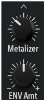
The Metalizer only affects the triangle wave. It increases the amount of higher and sometimes non-linear harmonics in the waveform through a process known as *wavefolding*. To understand how this works, visualize a standard triangle wave:
