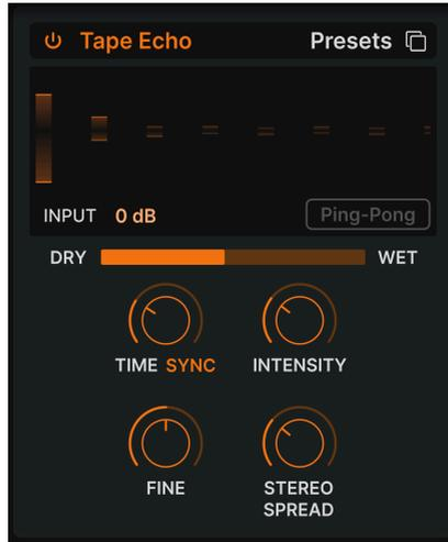
**Tape Echo** is a characteristic of early tape-based delay machines such as the Maestro Echoplex and Roland Space Echo. Input sounds are recorded to a loop of tape with one or more playback heads to create the echoes. Because tape loops can be unstable and shift in pitch and timbre, they produce an effect that is warmer and less precise than a digital delay.
