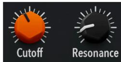
The **Cutoff** knob simply determines the frequency at which the filter begins reducing the volume of frequencies outside the permitted range. In lowpass or highpass modes, these frequencies are to one side of the cutoff or the other. In Bandpass or Notch modes, the cutoff is more correctly called a *center* frequency, as the knob sets the very center of the band that is either passed or rejected.
