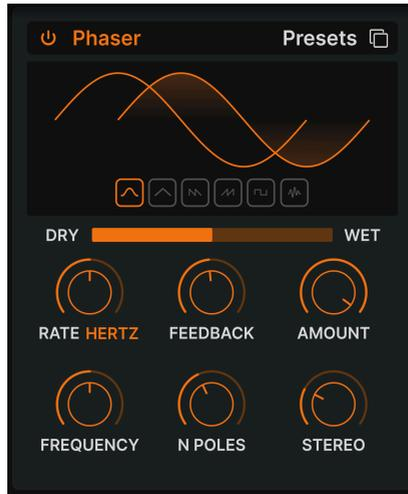
Phase shifting splits the incoming signal, changes the phase of one side, and recombines it with the unaffected signal. Modulation of this signal via an LFO results in a notch-comb filter that sweeps through the frequency spectrum, causing that familiar “whooshing” sound.
