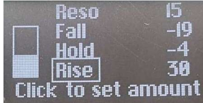
Macro Assign display for browsing modulation slots. The current slot is framed with a box.
