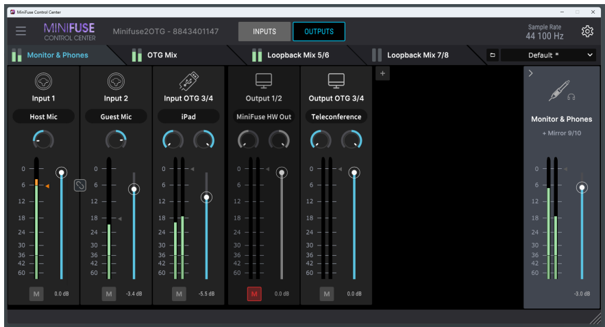
A simple mix of two microphones sent to a DAW on Loopback 9/10
