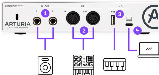
1 : TRS outputs to connect powered speakers or mixers/amplifiers
