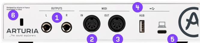
1. Outputs - these 1/4" balanced stereo outputs can be connected directly to active studio speakers or other devices such as amplifiers and mixers.
