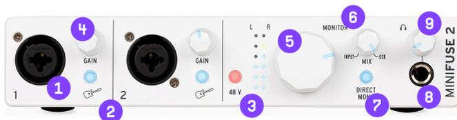
1. The **combo jack(s)** accept two different kinds of input - XLR and TRS - allowing you to connect a variety of microphones and instruments into the MiniFuse. The type of input is determined by the Guitar and 48V switches next to the input.
