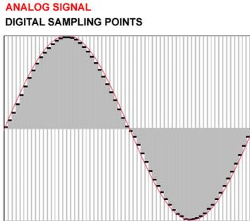
In the digital realm, analog audio signals are represented by discrete points in time, or "samples". When played back through a digital-to-analog converter, like those in computer soundcards, the digital samples are reproduced into a smooth audio signal. You can think of it like frames in a movie - each frame is a still snapshot, but when played back at a fast enough rate (24+ frames per second) our eyes perceive the sequence of static frames as continuous motion.
