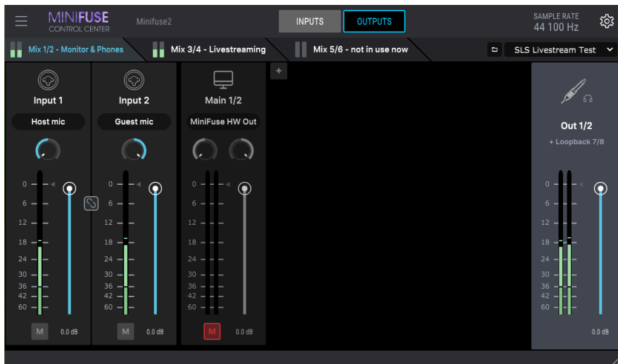
A simple mix of two microphones sent to a DAW on Loopback 7/8
