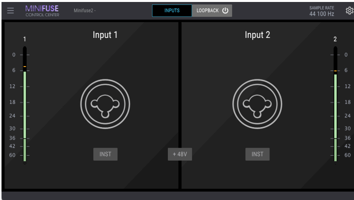
The Inputs tab in macOS, with metering and controls for the two Inputs
