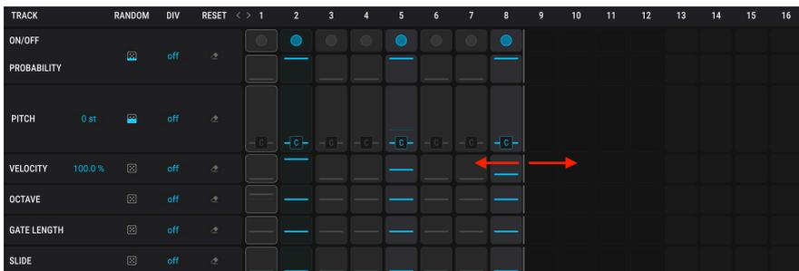
To change the length of the entire pattern, click and hover on the vertical grey line at the end of the last step in the pattern. The cursor pointer will change into a left/right arrow. Next, move the line horizontally and release it at the desired step length.
