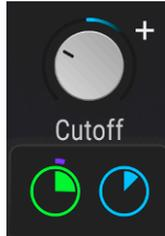
*Filter 1 cutoff is shown to be modulated by a Function (green) and a Macro (blue)*
