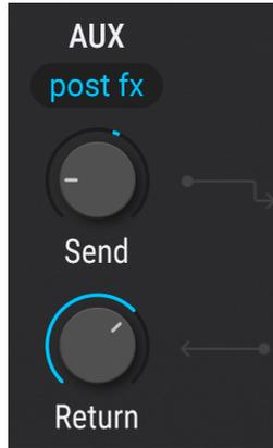
The FX Aux bus has three effect slots that are identical to those in FX buses A and B, so everything that you can do with one of those buses, you can do here. The difference is, where buses A and B operate as insert effects, the aux bus uses send-and-return routing. Send and return knobs appear here and in the [Play view \[p.70\]](#), as well as a Send Level knob in the main Synth view.
