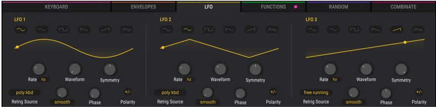
LFO stands for Low Frequency Oscillator, which is the most common source of modulations such as vibrato and tremolo in synthesizers. Think of it as a cycling up-and-down rhythm, which can do all manner of things depending on the destination(s) it's modulating.
