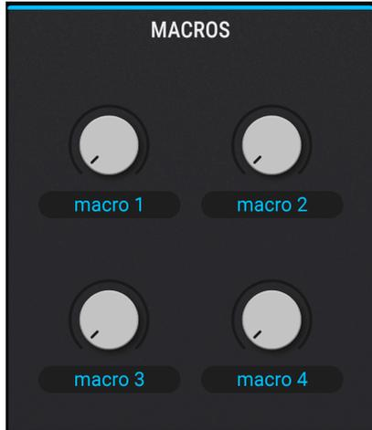
Macros are four unipolar knobs that can be assigned any number of modulation routings, including sidechains.
