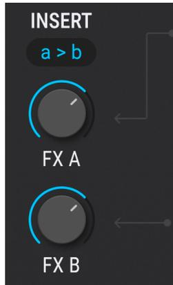
Use these controls to balance the output of Insert FX buses A and B relative to each other. The behavior is different depending on the configuration:
