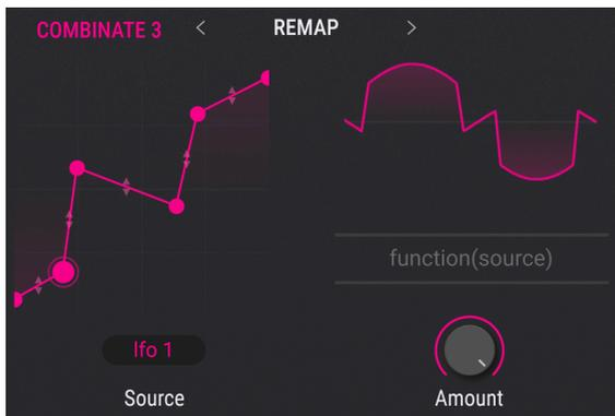
*The remap curve is at left; to the right is its effect on a sine wave*
