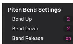
Click the gear icon next to the Pitch wheel to open the settings menu. Bend range can be set independently for Up and Down. For example, the upward bend can be set to +2 semitones and the downward bend can be set to -36 semitones. Whammy-bar solos are now within your reach!
