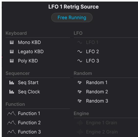
Here, you can select the source that causes the LFO to retrigger. That is, to start from the beginning of its phase. Note that the Engine 1 and 2 Grain options are available only when the Sample engine is selected as Engine 1 and/or 2, and its Granular mode is turned on.
