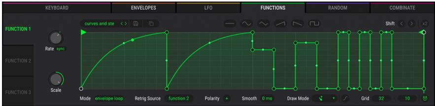
Each Function can contain up to 72 points, with independent levels and different curves between each point.
