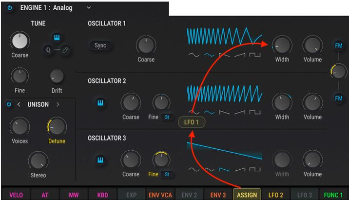
3. Release the mouse button. The assignment is made. The quick-edit knob will remain visible until you mouse away from the control.
