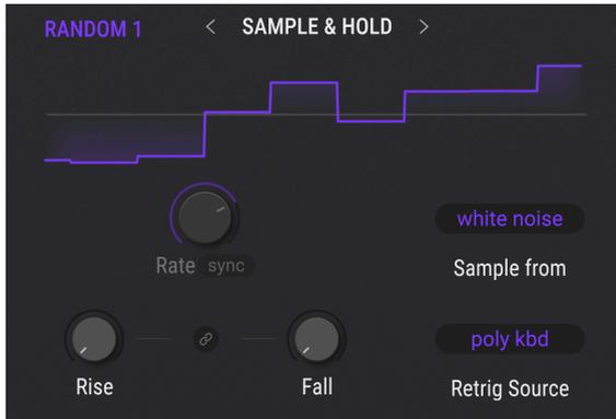
This term refers to sampling a source (most often a white noise waveform) at time intervals, then applying that value to a modulated destination.
