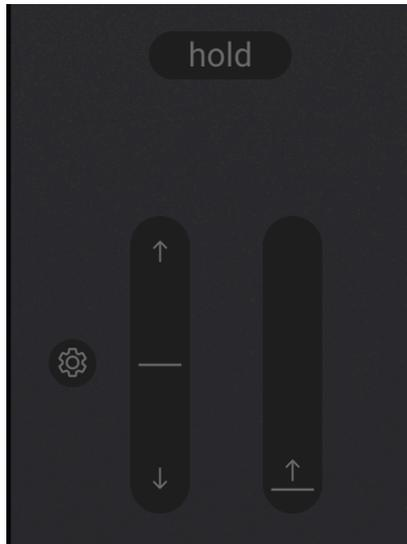
Located to the left of the virtual keyboard are the Pitch and Mod wheels. These wheels may be dragged up and down with your mouse. As you do they will perform the functions they have been assigned elsewhere in the user interface. They will also respond to the appropriate MIDI controller input.
