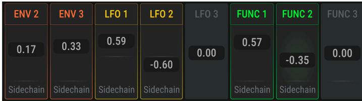
When the values are at zero the Mod source boxes are grey. As the values move away from zero the windows gain the color [p.215] of their modulation source type. "Sidechain" at the bottom means a Sidechain [p.227] can be added; if one exists, its name and level appear. Click one of those fields to change its setting.
