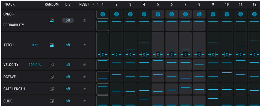
The largest section of the Seq/Arp window has six parallel tracks, each of which represents a different type of data that can be manipulated and sent by the Arpeggiator or the Sequencer, whichever is active.
