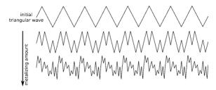
↑ The Metalizer can also affect all waveforms, not just the triangle, if its mode is set to "Level (All vaves") in the PolyBrute 12's settings. See the Metalizer mode [p.93] entry in Chapter 12 for details.
