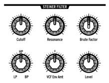
The Steiner filter defaults to *lowpass* mode in the Init patch, which means that anything below the corner frequency is allowed to pass; anything above it is gradually filtered out.
