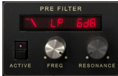
Rev Spring-636 Pre Filter section controls. Active switch shows the section is Off
