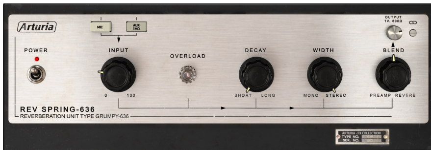
Rev Spring-636 Main Control Panel
