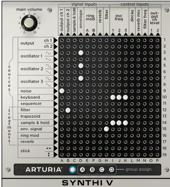
The Synthi's pin matrix is a brilliant piece of engineering! It gives you the massive power and flexibility of a modular synthesizer without the mess of cables or the massive size (the Synthi AKS was originally built into a small briefcase!) All you need is small plugs ("pins") to connect modules together. We will discuss the function of each module later in this chapter, but first let's first discuss how to use the matrix.
