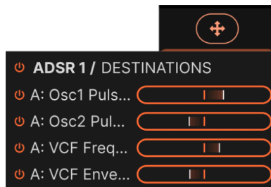
An ADSR assigned to both oscillators' pulse width plus the frequency and envelope amount of the filter, all in Layer A
