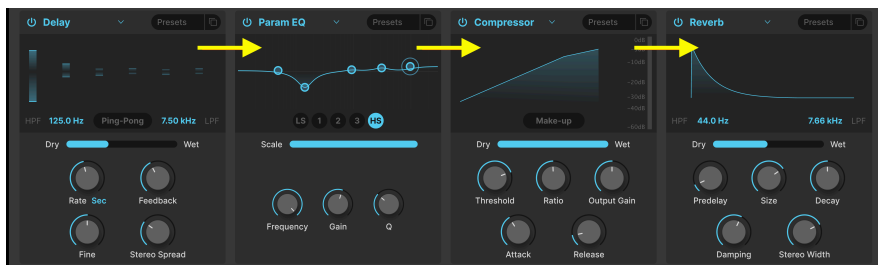
Synthx V effects are routed serially left to right
