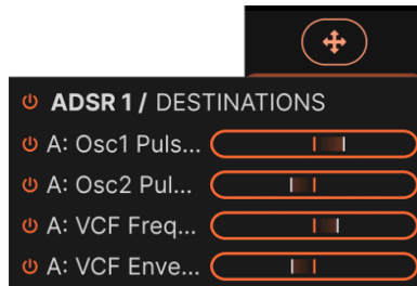
An ADSR assigned to both oscillators' pulse width plus the frequency and envelope amount of the filter, all in Layer A
