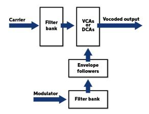
A vocoder contains two identical filter banks that cover specific bands throughout the audio spectrum, somewhat like a graphic equalizer. Vocoder V's filter bank uses 16 filters to create 16 frequency bands.
