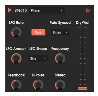
Phase shifting, first popularized in the late 1960s, adds a swirling, animated character to the sound. It works by splitting the incoming signal, modulating the phase of one split, and recombining it with the dry signal. This creates one or more notch filters, whose notch sweeps through the frequency spectrum, causing the phase shifter's signature "whooshing" sound. This stereo phaser models analog phasers, but also includes tempo synchronization.
