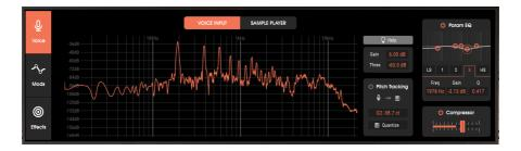
The Voice Input section controls the external signal coming from a DAW's track, or an audio interface's mic input in standalone mode. To simplify setting gain, the Visualizer screen shows the signal level and frequency spectrum.
