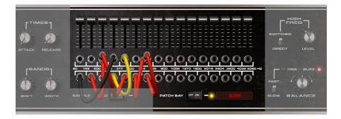
The Patch Bay allows for creative, innovative vocoder effects. In a standard vocoder, a Modulator band controls the same frequency band for the Carrier. With the patch bay, the analysis signals from any Modulator band (top row of jacks) can provide signals to articulate the Carrier synthesizer's bands (bottom row of jacks).
