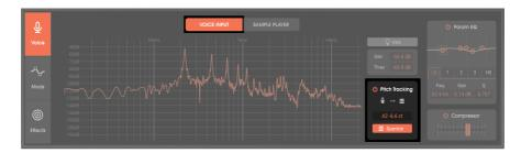
Vocader V can detect the pitch of a monophonic input signal, and use that to trigger the same pitch in the synthesizer keyboard. This allows playing the keyboard by singing, playing single-note lines on guitar, using wind instruments, and so on—exactly as if you had hit a key. This also means the Hold and Chord functions work with pitch-tracked notes, and pitch bend will bend the notes as well.
