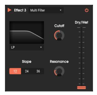
Multi Filter is a powerful sound-shaping filter, with five distinct filter modes, for sculpting frequencies at the output stage. It's much like the filters found in synthesizers.
