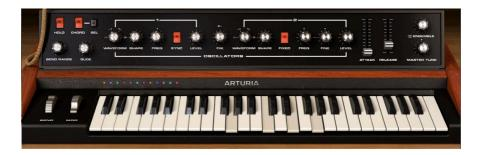
The Voice Input or Sampler Player interacts with Vocoder V's Carrier Synthesizer to create the vocoder effect. This two-oscillator synthesizer includes four waveforms, FM synthesis, an ensemble effect, hard sync, and glide (monophonic and polyphonic). To simplify vocoding, a Chord feature allows playing any of several chords, or a custom chord, from a single note. Additionally, a hold option can hold a chord or single note indefinitely, while you modulate it from the input signal.
