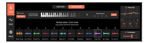
The Sample Player feature is unique to Vocoder V. It stores up to 12 mono or stereo audio files of essentially unlimited length, which play back monaurally. Thus, these samples can provide audio to the vocoder section without needing to route a microphone or other sound source to the vocoder. This makes it possible to play Vocoder V more like a traditional keyboard instrument. Also, samples are saved with presets, so that recalling the preset recalls the samples.
