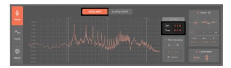
Gain (-36 dB to +24 dB). Set this for the optimum input level to Vocoder V. Ideally, peaks will reach, but not exceed, -18 dB. There is another level control in the vocoder section to set the modulation level; think of that as the master level control, and Gain as the preamp gain control.
