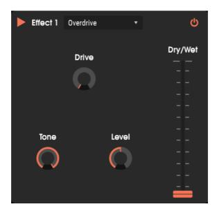
Overdrive adds enough gain to the input so that it runs out of headroom, which cause the input to clip and distort. This introduces harmonics that add a harsh edge to sounds, and is similar to an overdrive pedal for guitar.
