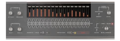
The 16 sliders control the output levels of the Carrier synthesizer's bands. Use this feature to reduce the levels of bands whose frequencies conflict with other instruments, or increase levels with bands that help increase intelligibility.
