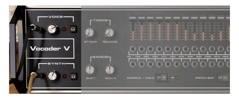
To optimize levels going into the Vocoder, both the Modulator (Voice) and Synth (Carrier) have level controls with a range of -75 dB to O dB gain. Don't set the levels too low, but avoid lighting the red clipping indicator to the right of either level control.
