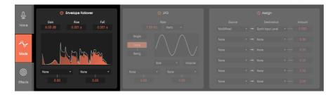
The Envelope Follower control signal represents the amplitude of either the Voice Input or Sample Player from the Voice section, after it has gone through the Param EQ and/or Compressor effects (see section 5.4). The Envelope Follower graphic shows the waveform in orange, while the white line shows the result of any smoothing added by the Rise and/or Fall controls (see next). A power on/off switch enables or bypasses modulation from the Envelope Follower.
