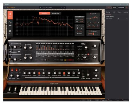
The toolbar at the top of the interface provides (from left to right) a menu for file management, setup, and help, as accessed by clicking on the three lines at the upper left. The middle section accesses the Library and preset Browser. Additional buttons to the right choose between the Voice or Sample Player input; the Advanced button shows or hides the Advanced panel, and the Gear icon opens the flyout.
