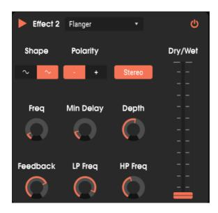
The Flanger effect is based on the same general principle to the Chorus effect above, except that the delay time tends to be much shorter (as low as 0.001 ms). The extremely short delay time produces a "comb filter" effect that sweeps up and down through the harmonics of the original signal.
