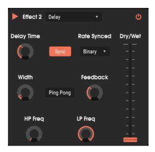
Delay can increase a sound's spaciousness by copying the sound at the input, and playing it back later at a reduced level—what's called an echo. Compared to reverb, this gives a more focused, less complex sense of space. Another application is setting delay to sync with a song's tempo, which can provide a rhythmic counterpoint that emphasizes a groove.
