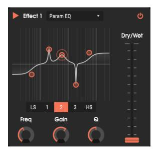
The parametric equalizer is a versatile way to adjust frequency response, because it can boost (make more prominent) or cut (make less prominent) specific ranges of the frequency spectrum. This kind of EQ is suitable for broad tone-shaping, or precise, surgical fixes. The Param EQ has five stages: Low Shelf, three fully parametric stages, and a High Shelf. Each has the same three associated controls.
