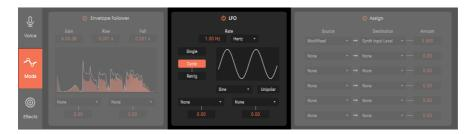
The LFO is polyphonic, so every voice in the Carrier has its own LFO, controlled by the parameter values in the LFO section. The LFO provides six waveform shapes, which can run continuously or be triggered in various ways. The LFO display shows the selected waveform, and how it's affected by the following controls.
