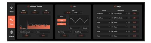
The Mods section provides control signals that you can route to several destinations in the vocoder and synthesizer sections.
