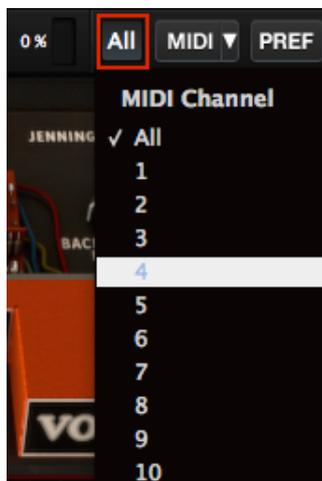
If you select a channel here, only data arriving on that MIDI channel will be received. So when the Global channel matches the MIDI channel for one of the three instruments (Upper, Lower, or Bass) that sound will be able to receive MIDI data. When it lands on a channel outside of those assignments, the sound of the Upper instrument will be available to incoming MIDI data.
